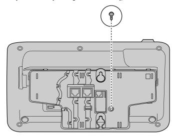
**3.** Connect the cables to the unit, and run the cables through the wall mounting adaptor, as shown in the illustration below.
