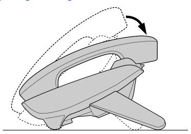
**1.** Tilt the stand in the direction indicated while pushing the PUSH mark with both hands as shown until it locks into the low position (**3**).
