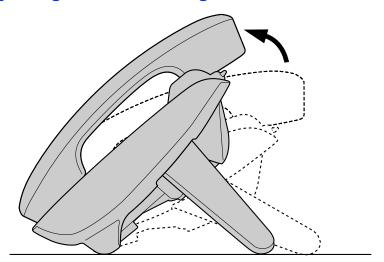
1. Tilt the stand in the direction indicated while pushing the PUSH mark with both hands as shown until it locks into the high position (A).
