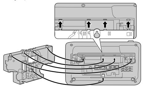
2. Fasten the wall mounting adaptor to the base with 1 screw. (Recommended torque: 0.4 N·m [4.08 kgf·cm/ 3.54 lbf·in] to 0.6 N·m [6.12 kgf·cm/5.31 lbf·in])
