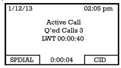
4. After the call ends and if the queue has wrap up time configured, the phone displays the wrap-up period information. Agents can receive and place calls while in the wrap-up period. The agent ends the wrap up by pressing the CANCEL soft key button.
